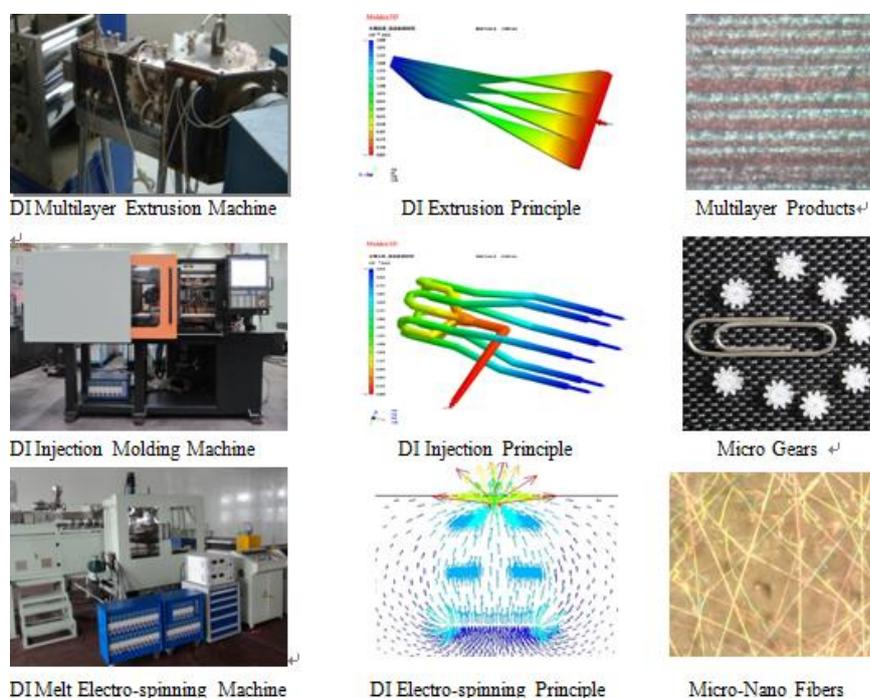
FIGURE 1. Equipments, principle, and product of melt DI injection molding, DI nano-composites extrusion molding and melt differential electrospinning.
