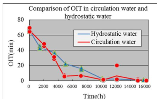
Figure 2 OIT changes with testing time as a parameter of circulated and hydrostatic hot waters.
