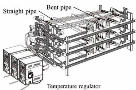
Figure 1 Hot water circulation test.
