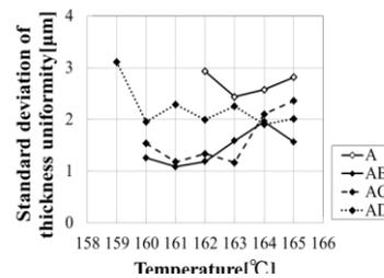
Fig.2 Thickness uniformity & stretchable temp.
