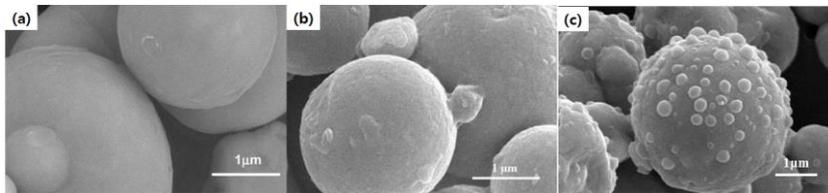
Fig. 1: SEM of magnetic hybrid particles: a) CI/PMMA, b) CI/cross-linked PMMA and c) CI/PS
